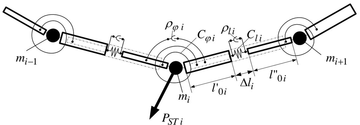
**Fig. 4. Discrete model of the elementary component of the rod**
