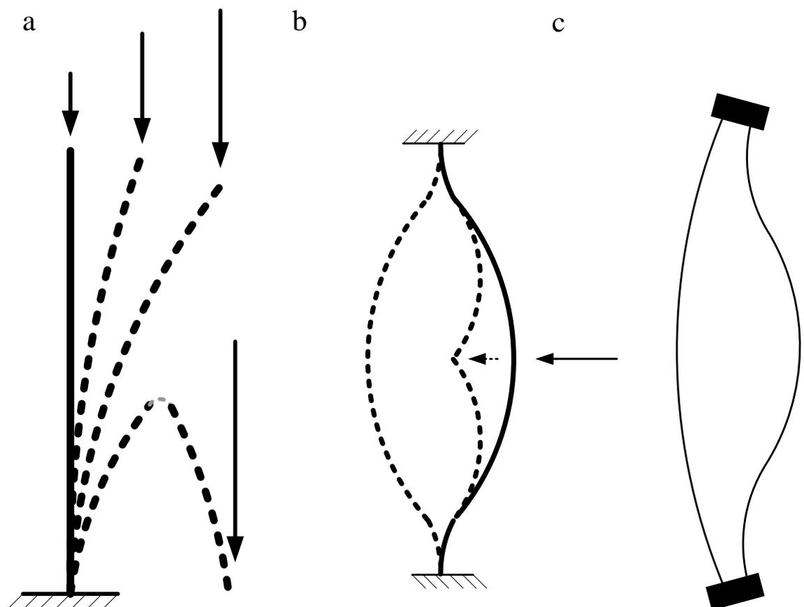
**Fig. 8. Loss of stability (and "breakdown") of a rod with axial load – "Euler task" (a); passage from one steady state to another (b); the bend of two parallel rods (wires), pinched from both sides (c)**
