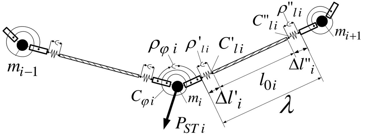
**Fig. 2. Discrete model of the elementary component of rope**
