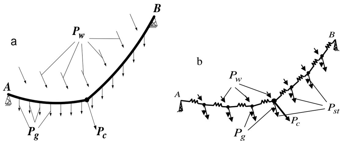
**Fig. 1, a) - Rope, sagged in the gravitational field, is loaded with wind action and concentrated load; b) - its discrete model**
