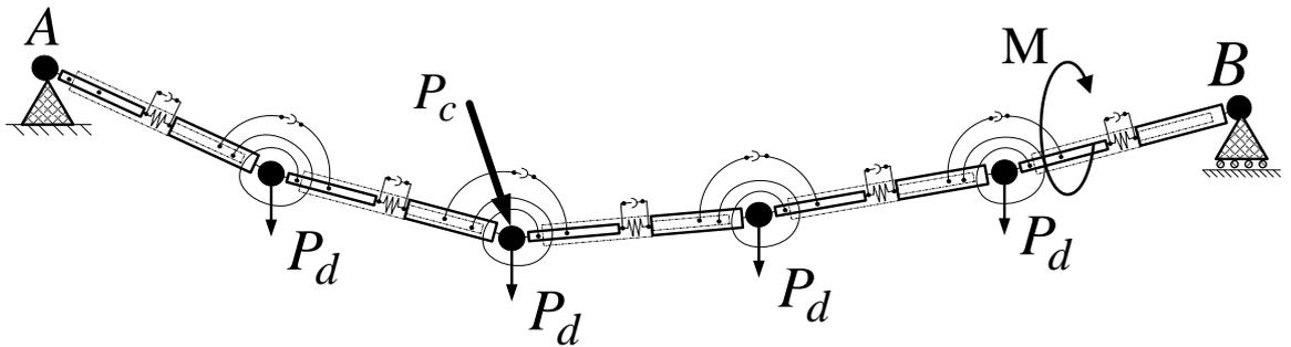
**Fig. 5. Discrete model of a beam with concentrated load**
